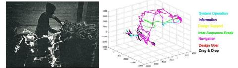
*Figure 5 – Original Gilbreth Chronocyclegraph (left) and VR Chronocyclegraph (right)*
